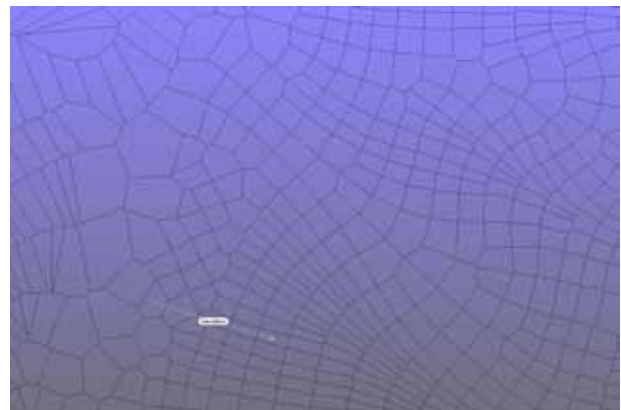
Initial tessellation based on water flow lines and contour lines
