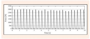
Figure 1. Example of a vertical jumping force record due to test subject 3 continuously jumping at 2.4 Hz jumping rate.
