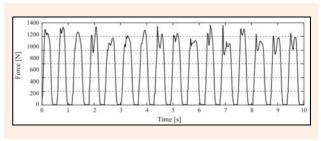
Figure 2. Force history generated by test subject 6 while jumping slowly at 1.6 Hz jumping rate.
