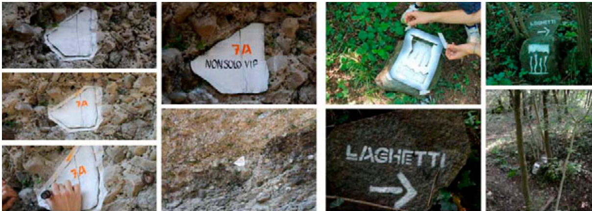
Fig.5 – On-site test session photos: identification sign for a single climb route and directional sign along a trail realized by using water based paint-spray and a black pen marker.
