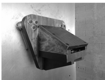
Figure 5. Example of rigid target structure for birdstrike.
