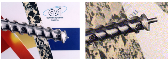
Fig. 3 Some details of the Drill Rod with Sampling Tube retracted (drill mode-left) and extracted (sampling mode-right)
