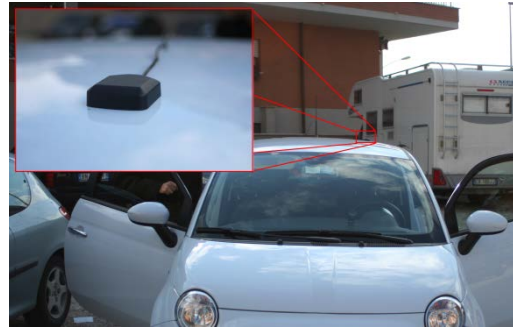
Figure 1. The u-blox antenna positioned on the rooftop of the car.
