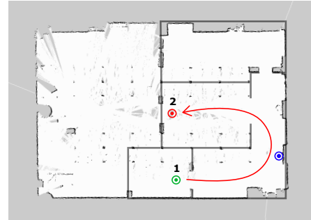
Figure 7: Schema of Exp. 1b: The user moves from Room 1 (in green) to Room 2 (in red) while being approached by the mobile robot. The robot (starting from the blue point) has to identify and approach the user while this moves across different rooms.
