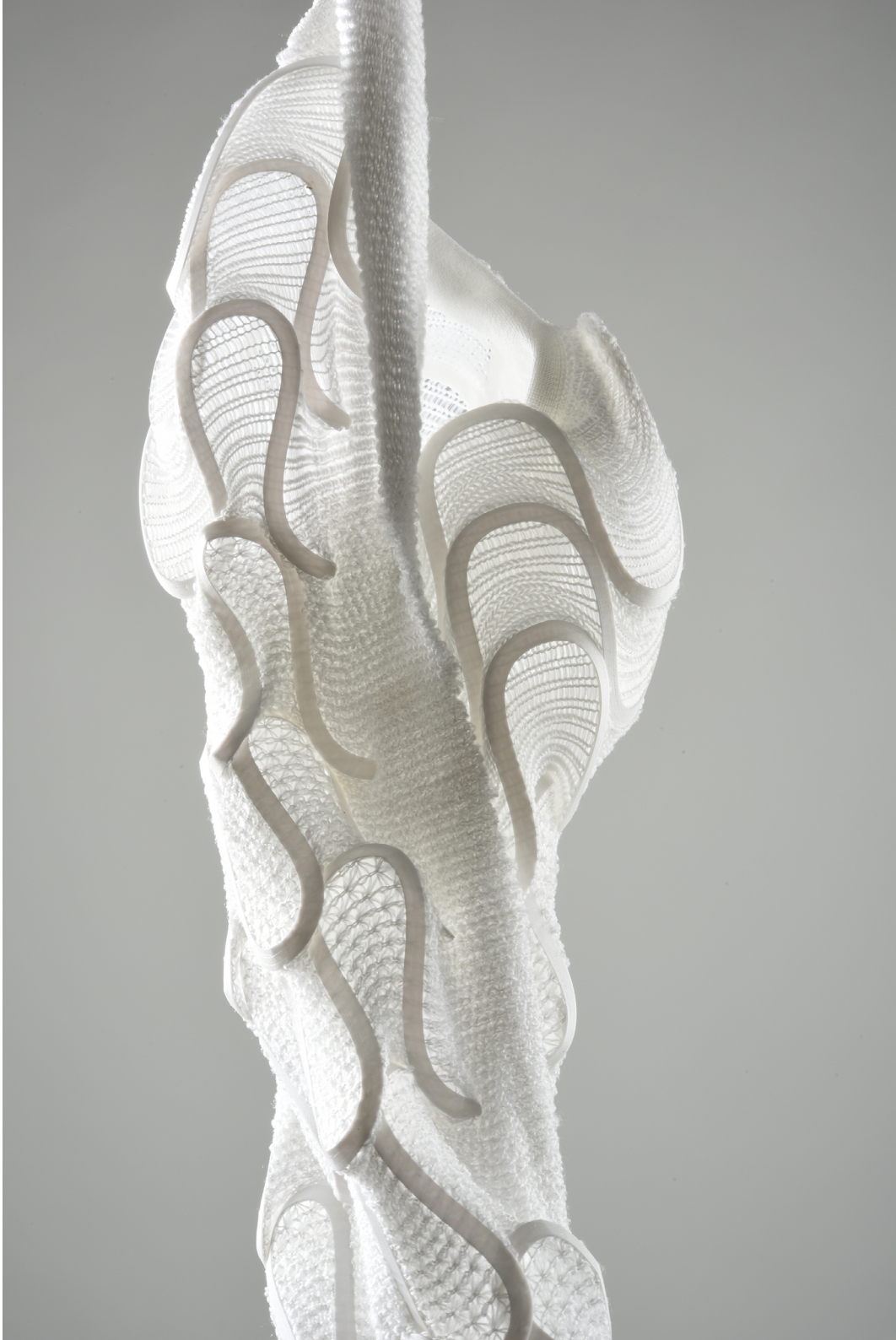
FIGURE 1. D printing on a custom knitted fabric with tuck stitch and drop stitch pattern (Agata Kycia)
