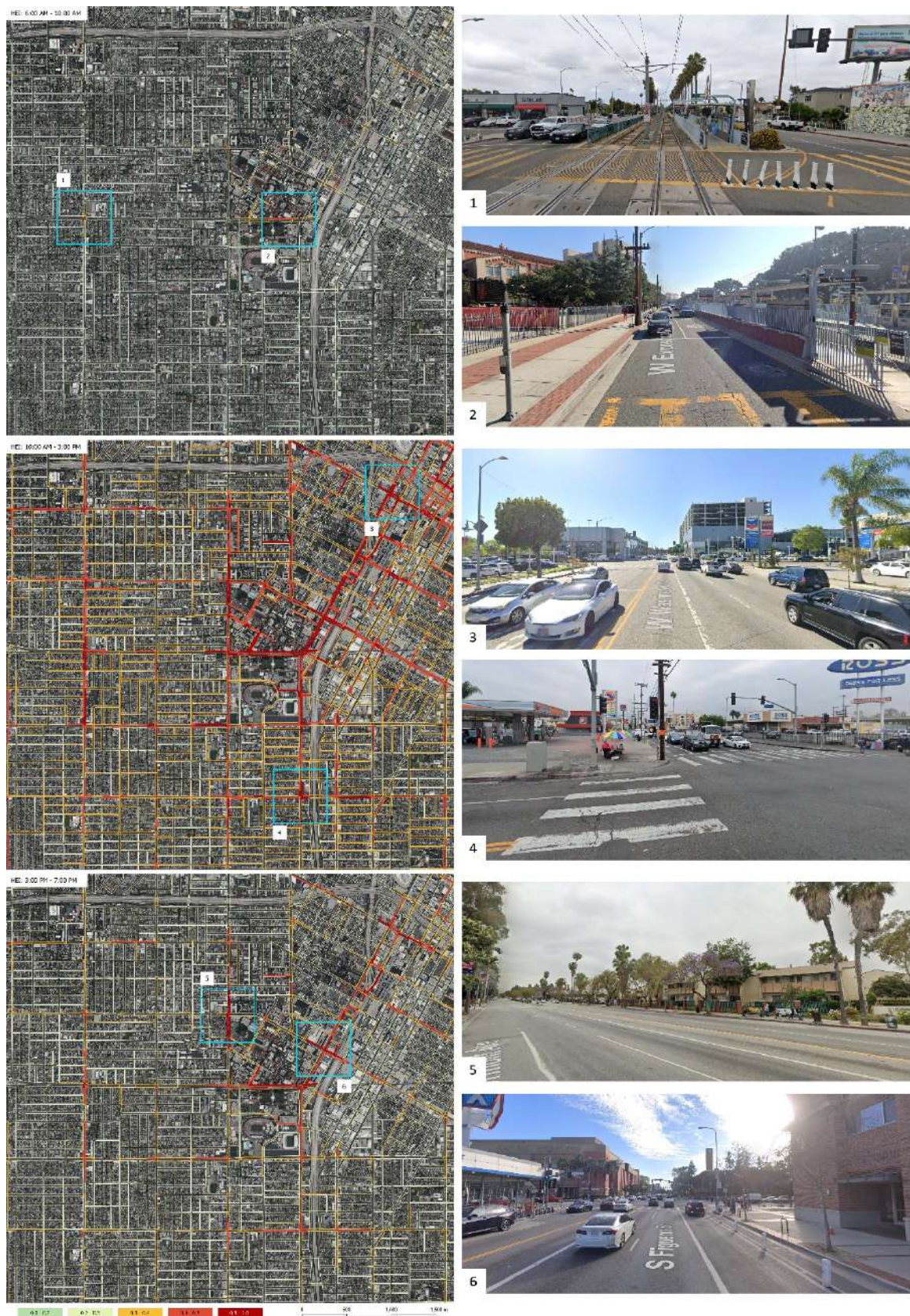
Fig.2 Sidewalk-level HEI: morning (6-10 A.M., top panel), midday (10 A.M.-3 P.M., middle panel), and evening (3-7 P.M., bottom panel), with corresponding street-view insets (1-6) showing how urban features shape pedestrian heat exposure
