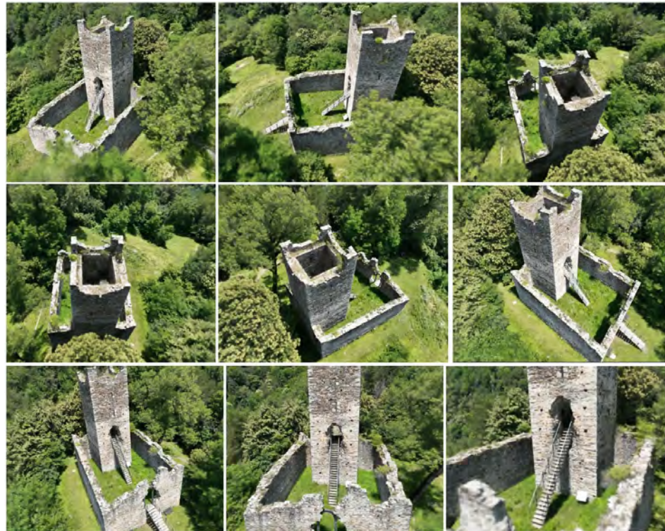
Figure 1. Frames of a rendered video created using NeRFs and a set of oriented images. The fortified construction is Mancapane Castle. The frames were generated with Nerfstudio using a set of images oriented with Metashape.
