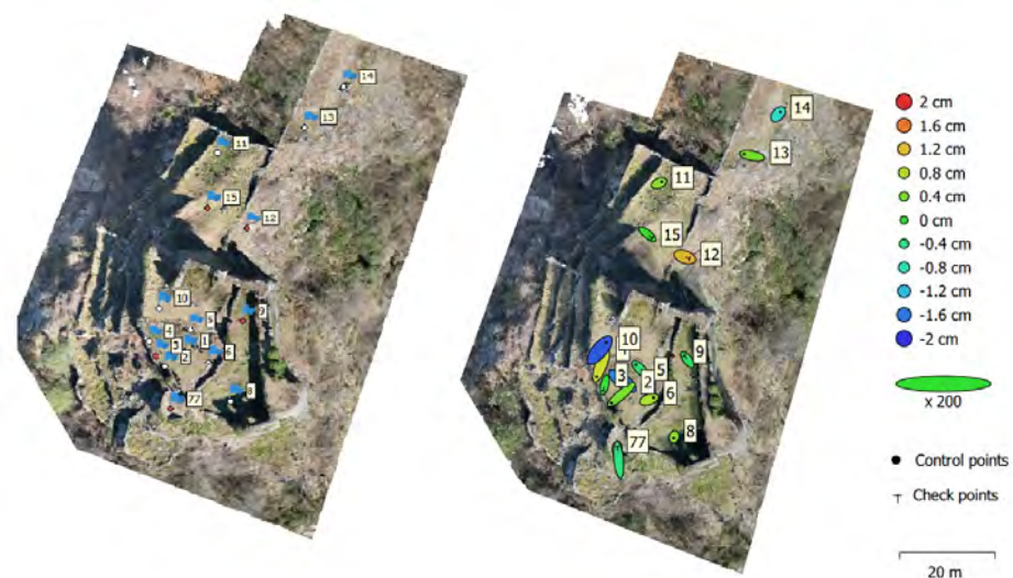
Figure 9. Vogogna dataset: position of GCPs (white) and CPs (red) on the left and position residuals represent as error ellipses on the right.
