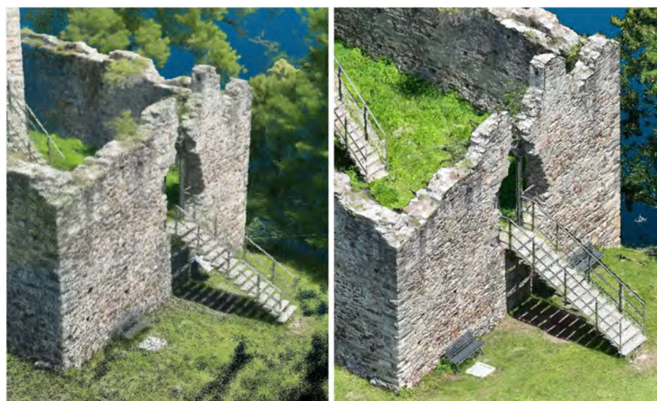
Figure 18. Point clouds produced with Nerfstudio (left) and Metashape (right) using the same set of images.
