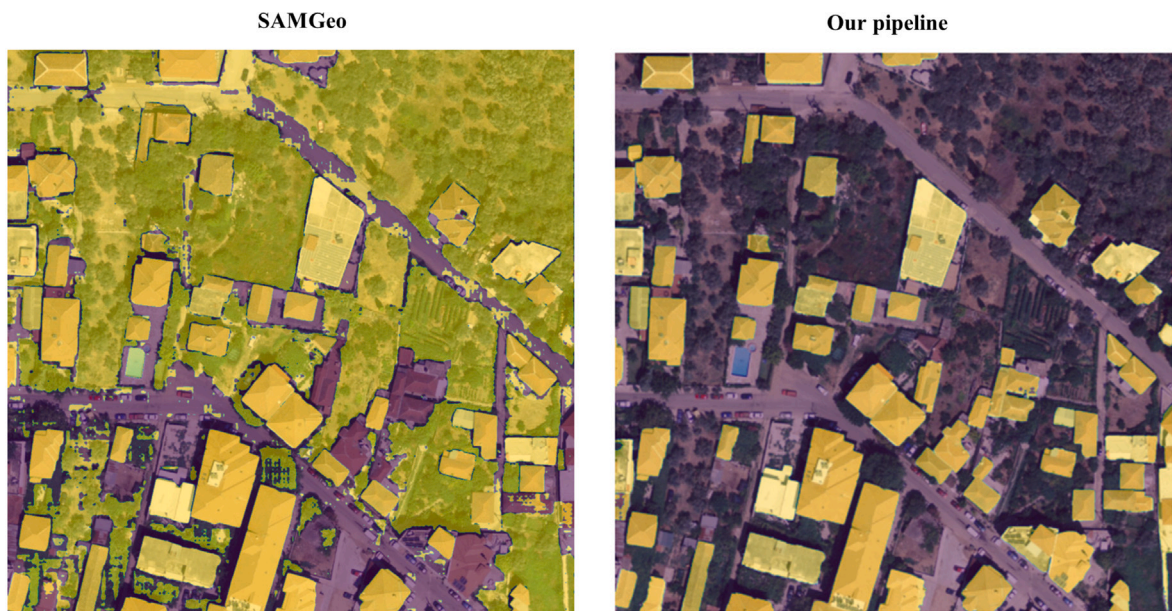
Fig. 11. "The segmentation masks of applying the SAMGeo and our pipeline for the prompt Roof".
