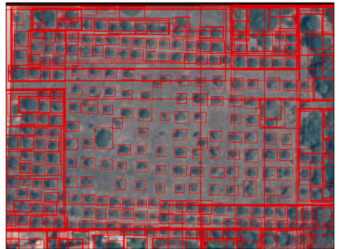
Fig. 4. Grounding DINO object detection with 0.1 hyperparameter values for the prompt “trees”.
