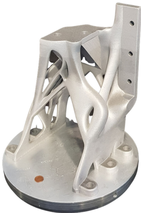
Fig. 1 Example of a medium sized component produced by LPBF in AlSi7Mg alloy. The build plate diameter is 300 mm, while the part height is 385 mm
