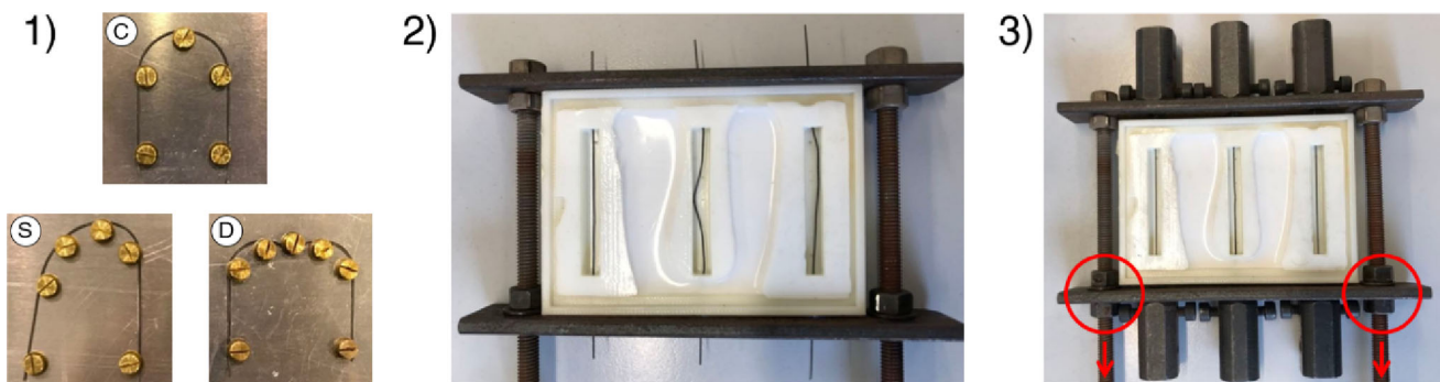
Figure 1 Fabrication process of the composite samples. 1 The wires are shape set with custom jigs and subjected to thermal annealing. 2 The wires are put in a silicone mould within a metallic jig. This already partially straightens them. 3 The wires are blocked with metallic crimps, to fix them to the jig, and are
