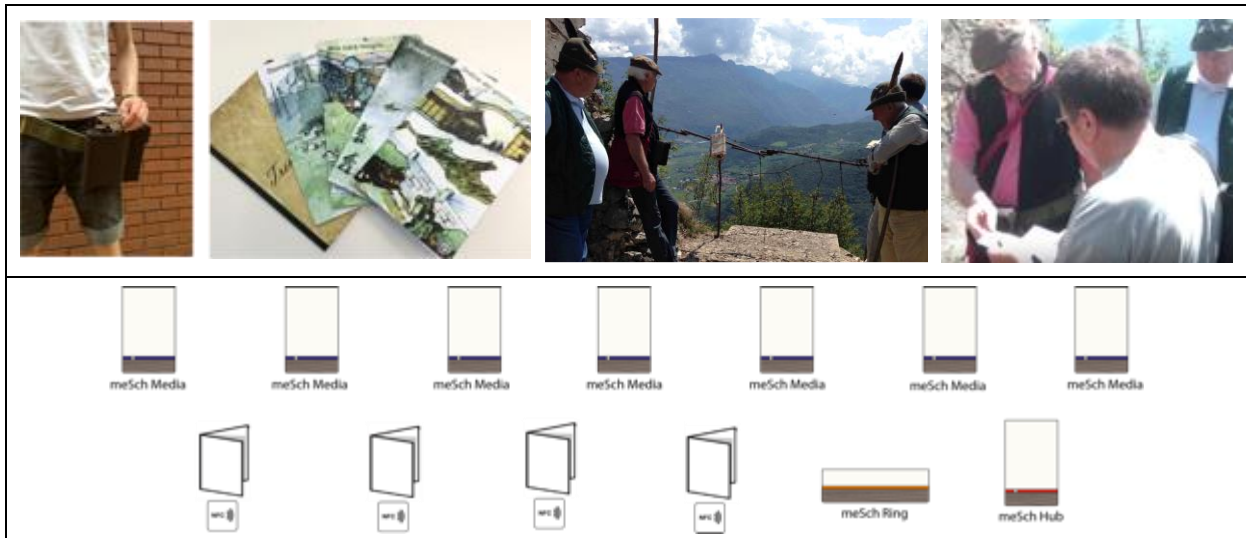
Figure 2. The interactive belt designed to be used while trekking in the Italian Alps visiting the trenches of WWI. (top row) The belt and the thematic cards are worn by the visitor while the Bluetooth-augmented loudspeaker marks the point of interest. Visitors in group negotiate what to listen to next. (bottom row) Each of the seven places is marked by a lantern that conceals a Media node that plays the sound / stories; the four cards are NFC tagged; the belt hosts both the Ring to read the tags and the Hub to communicate with the Media nodes.
