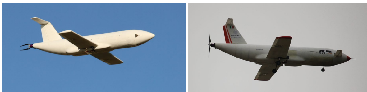
Figure 2: The Aether platform in two- (left) and three-surface (right) configuration, during flight tests.
