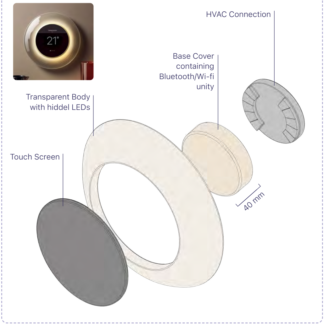
Figure 48. Drawings and main parts of the wall-mounted design.
