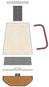
Base containing pcb, power connection and control buttons
