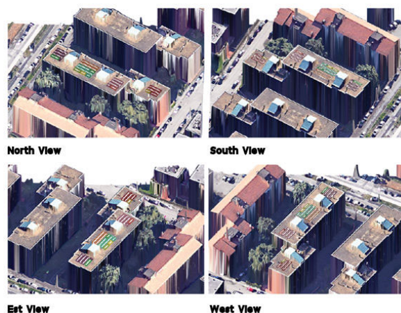
Figure 3. Design and simulation of condominium in OpenSolar software.
