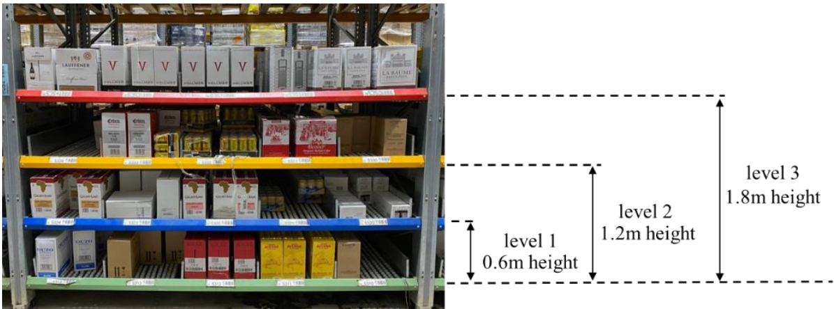
Figure 2. Sample front view of the high-density flow-rack storage system
