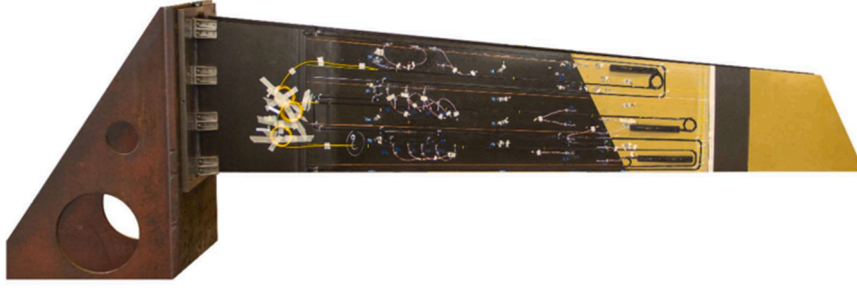
Fig. 8. Test sample and its supporting system (view from the upper skin side).
