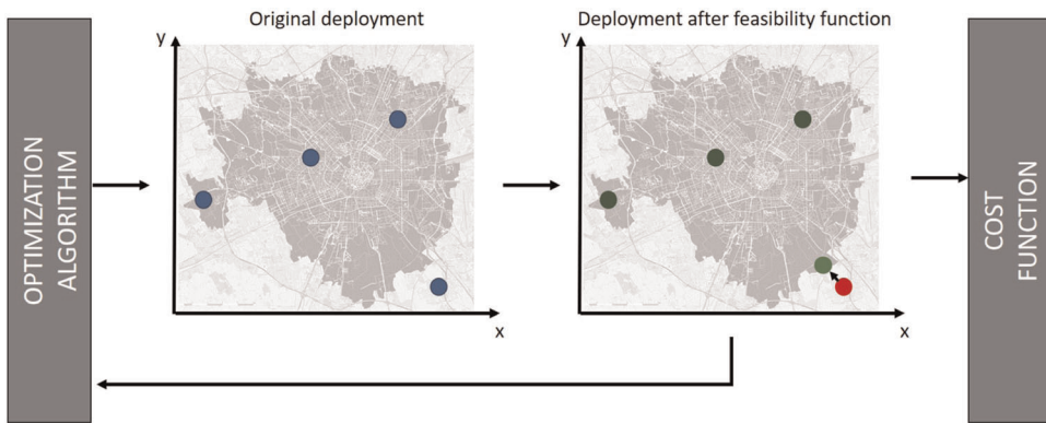
FIGURE 5 Optimization process: effect of the feasibility function. All the charging stations outside the urban area are mapped to the closest feasible position: the obtained solution is used for the cost function computation and it is feedback in the optimization loop [Color figure can be viewed at wileyonlinelibrary.com ]
