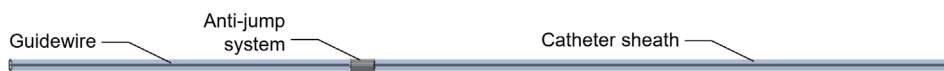
FIGURE 4 | Delivery system including the guidewire, the catheter sheath and the anti-jump system.
