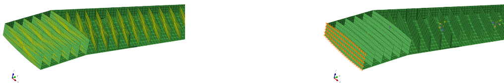
(a) Coupling constraints applied on each rib of the model, in yellow.
