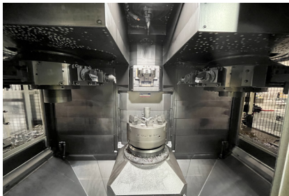
Fig. 2. "Lathe Machine 1" with two revolvers (Left: Revolver-1, right: Revolver-2)
