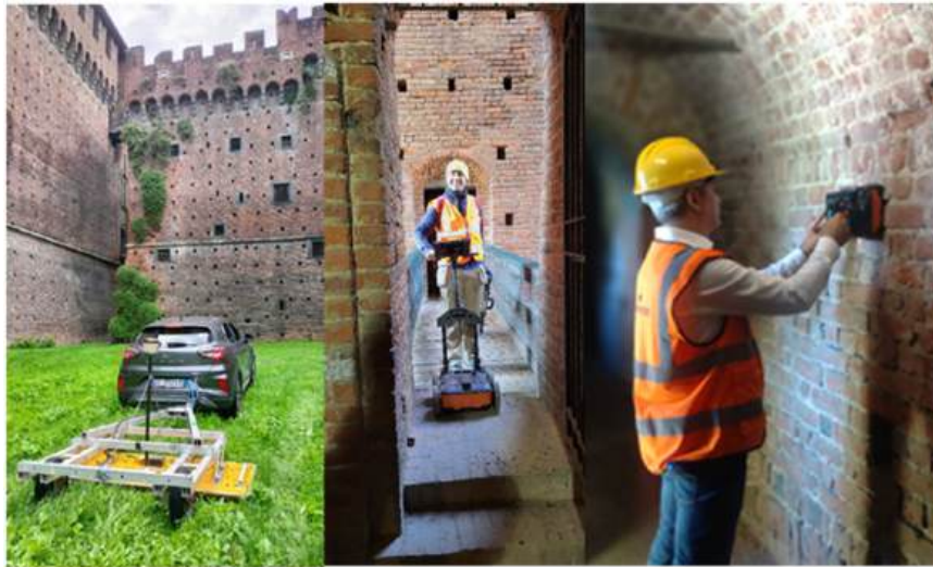
Fig. 6. GPR systems employed during the survey at Castello Sforzesco. From left to right: the Kontur array; the GSSI UtilityScan and the GSSI Flex NX.
