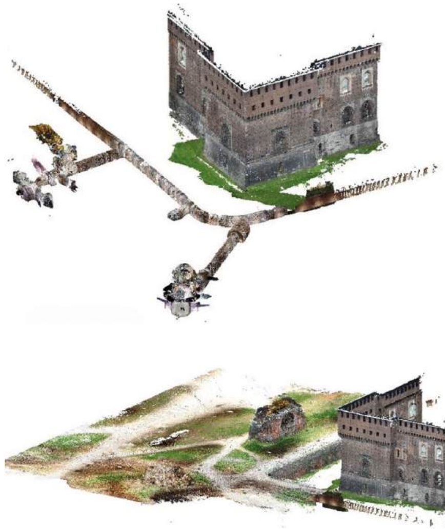
Fig. 3. Views of part of the point cloud implemented for the development of the 3D model.
