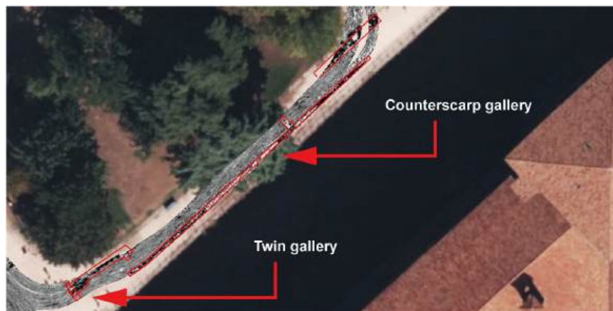
Fig. 9. The depth slice image shows the parallelism between the known counterscarp gallery and the unknown "twin" gallery.
