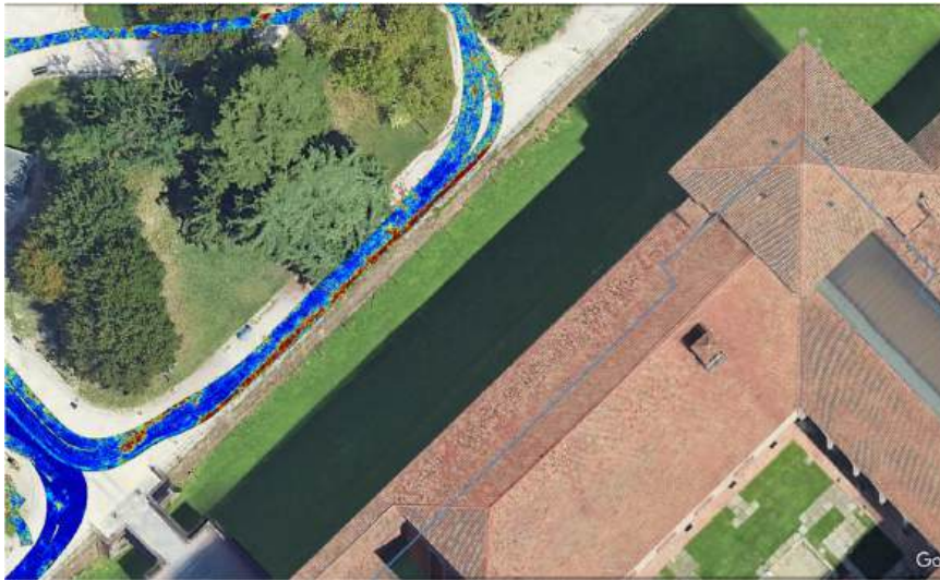
Fig. 17. 3D GPR data view of the counterscarp and “twin” galleries.
