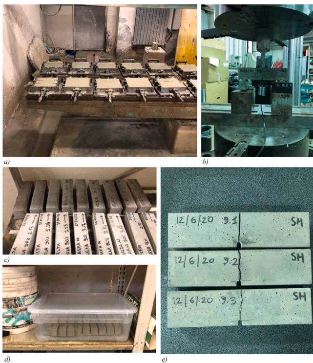
Fig. 17. Healing of matrix cracks — Experimental investigation (a) casting, (b) pre-cracking after 45 days in moist chamber, (c) curing with exposure conditions A, (d) curing with exposure conditions DW1 and DW2, (e) broken healed samples after 3-point bending tests.
