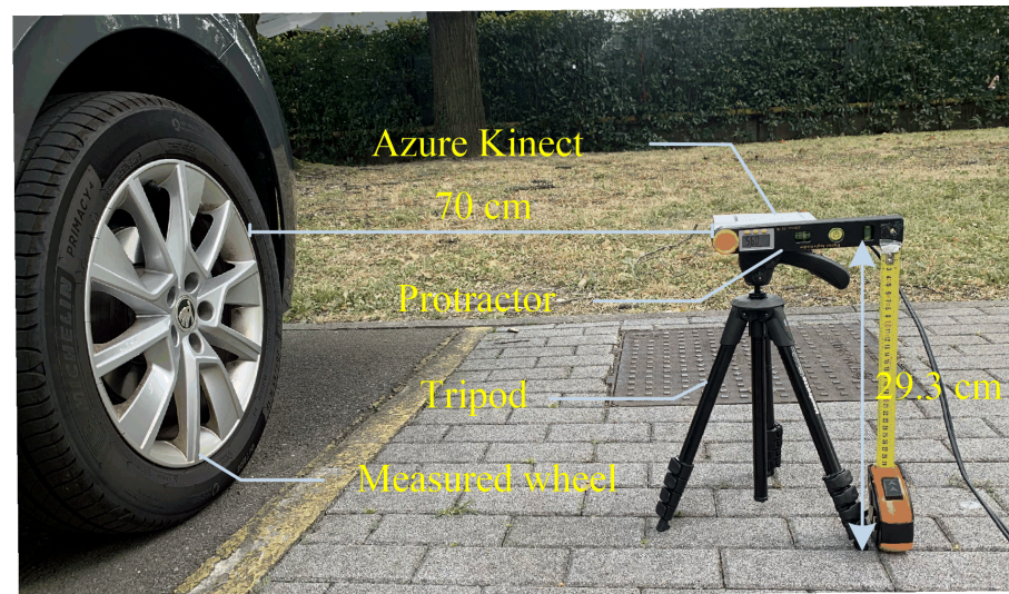
Figure 7. Schematic diagram of the measurement platform.
