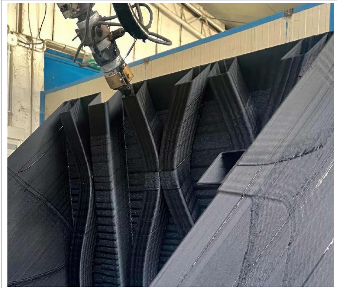
Fig. 3 3D printing of the component (Credits: The Authors, 2024).
