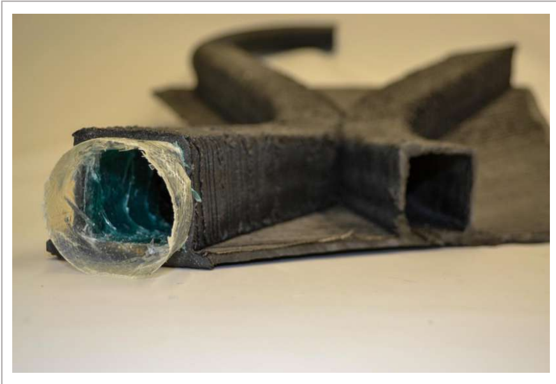
Fig. 2 Details of hollow ribbed panels reinforced with composite material (Credits: The Authors, 2024).
