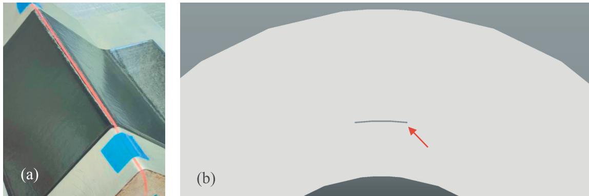
Fig. 2. Focus on the defect: (a) Teflon placement during lamination; (b) zoom on the location.
