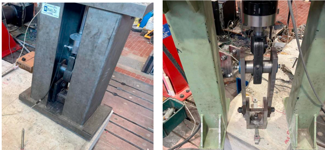
Fig. 3. Test setups: on the left confined and on the right unconfined tests
