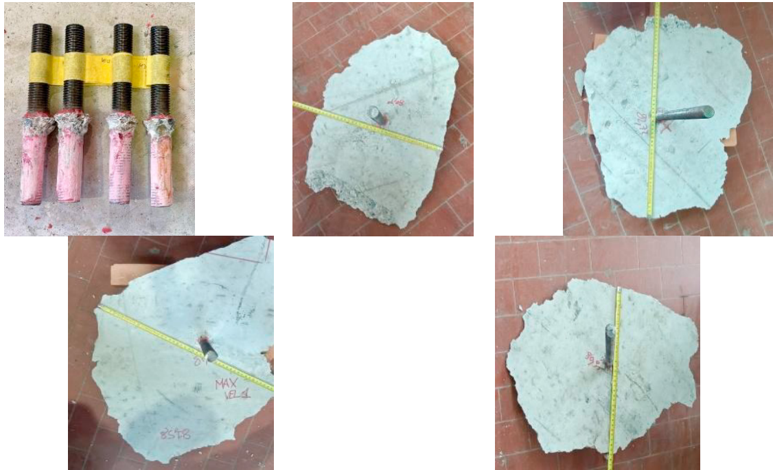
Fig. 6. Confined and unconfined failure modes
