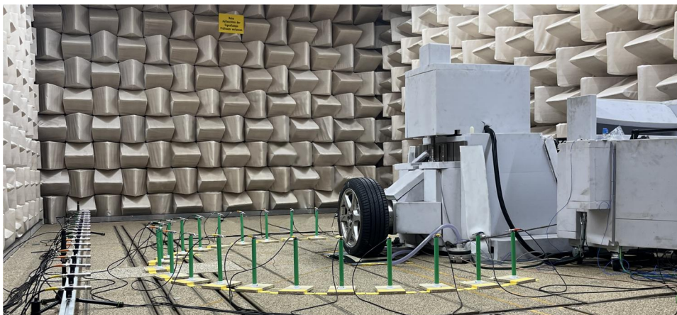
FIG. 2. Tire test rig used for indoor noise measurements in the semi-anechoic chamber.
