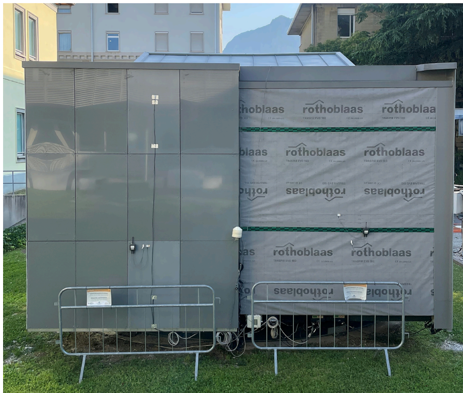
Fig. 8. Front view of the living laboratory, on the left side the monitored OVF and on the right side the wall without the OVF technology;
