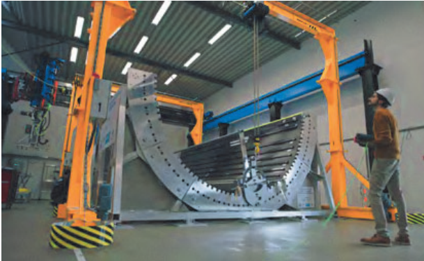
Figure 7: An automated manufactured lower shell of the fuselage of the future (Credits: Oculus Film)
