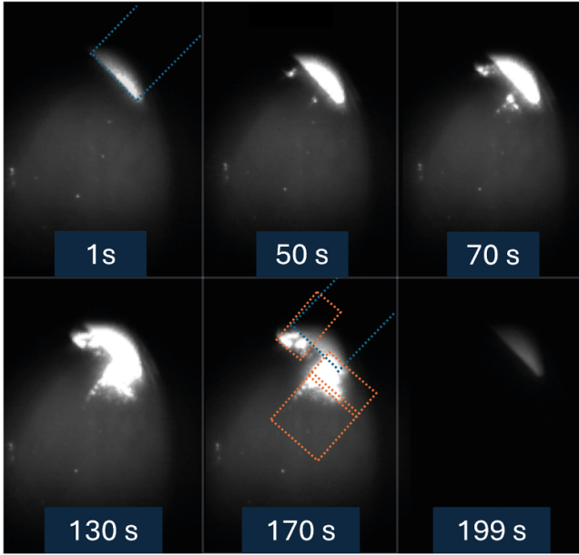
Figure 12. IR camera stills from the exposure of target set M(P). The blue dotted lines outline the position of the W sputtering plate, which is heated and therefore glows. The orange dotted lines indicate the positions of different targets in the clamping ring assembly. The bright regions increase in size over time, and are indicative of poorly adhered layers which are then badly cooled and thus strongly heated by the plasma. At 199 s the bright regions have disappeared, showing that these regions have flaked from the surface.
