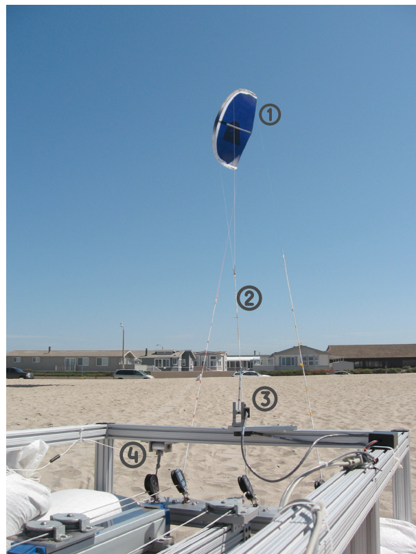
Fig. 2. Experimental setup of UC Santa Barbara 12m 2 Prototype. (1) Kite, (2) Tethers, (3) Sensor estimating elevation \theta and azimuth \phi , (4) One of the three tether force sensors
