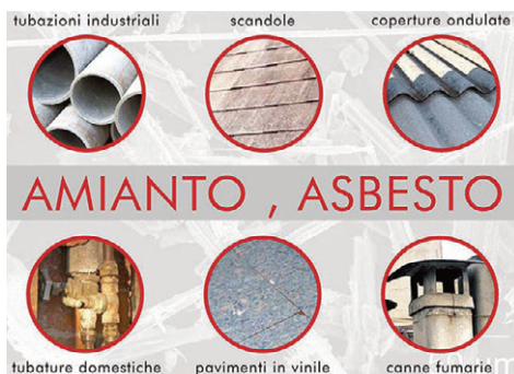
Fig. 7 | The presence of asbestos in buildings (credit: infobuildenergia.it).
