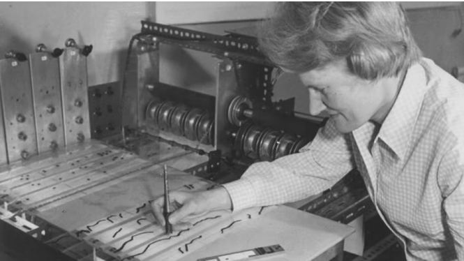
Fig. 3. Oramics Machine with a neume cutting block, operated by Daphne Oram.
