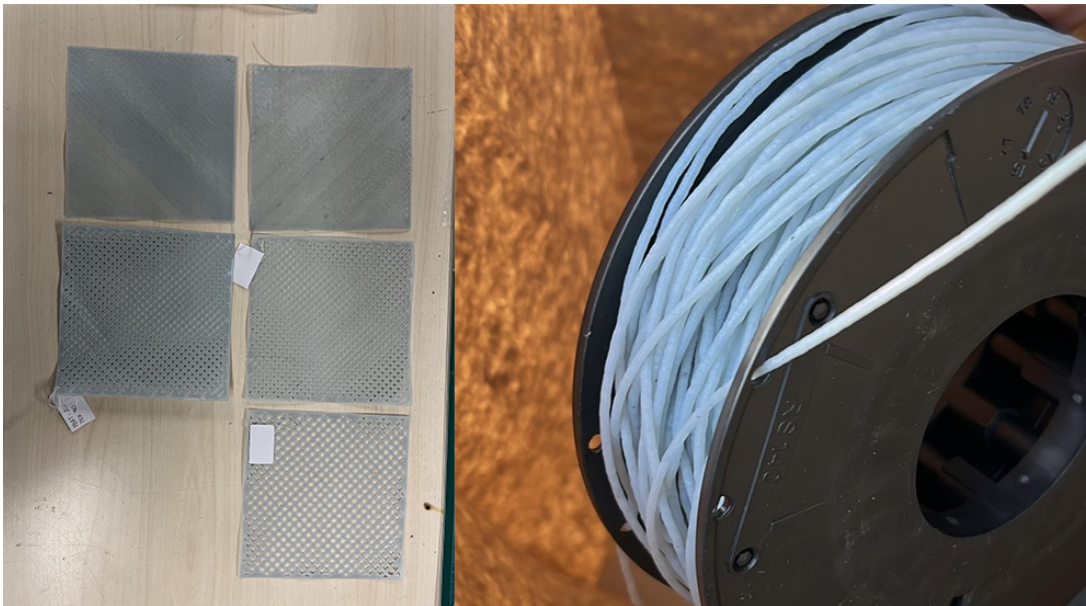
Fig. 3 Fiber2filament process – Cotton starter, filament extrusion, and sample printing. Credits: Flavia Papile.
