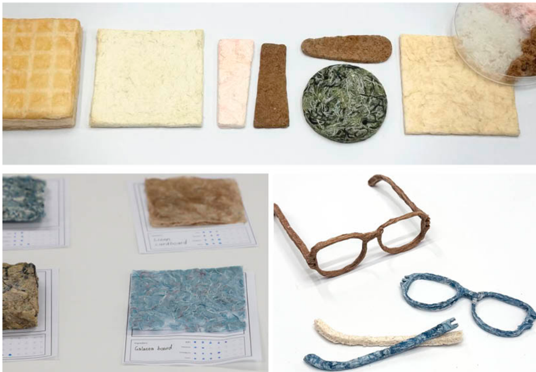
Fig. 5 REFABbio - BIOCOMPOSITE SAMPLE FROM TEXTILE WASTE - TEXTILE WASTE COURSE & MATERIAL COOKBOOK. Credits: Nicla Guarino & Ziqian Yu.
