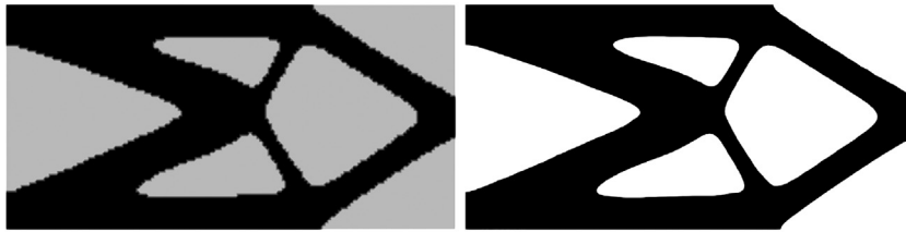
Fig. 1. CLC. Output of the level set method on a fixed mesh: function \chi_{\varphi,h} (left) and final layout \bar{\Sigma}_h (right).
