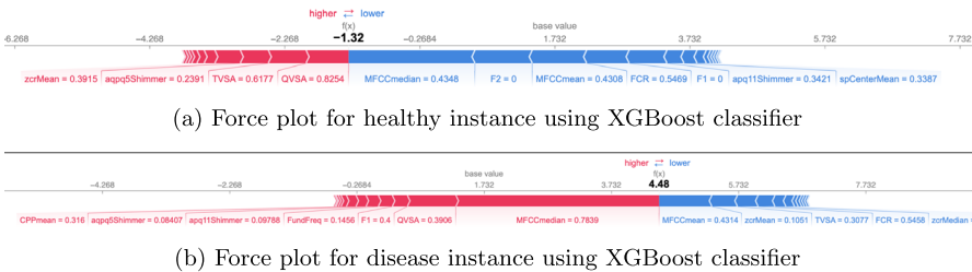
Fig. 7 Example of force plots for local explainability in healthy (a) and disease (b) instances. In a, a final prediction of -1.32 , below the base value of 1.732 , is shown, resulting in a healthy classification. In b, a prediction of 4.48 , significantly above the base value, indicates a disease classification. Both force plots highlight MFCCmedian, MFCCmean, and QVSA as key features, demonstrating their influential positive and negative contributions to the classification
