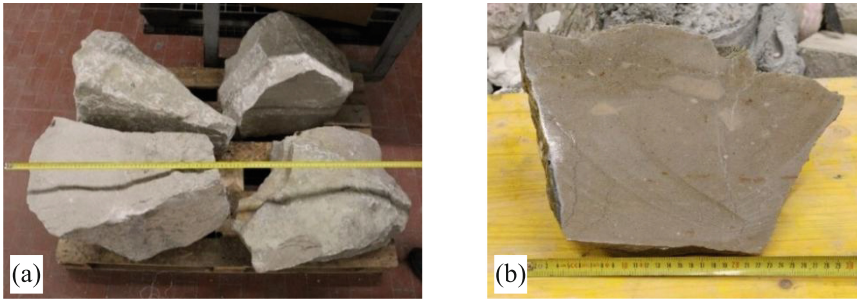
Fig. 2. a) Four Saltrio stone blocks extracted from the Salnova quarry; b) visible microfractures, inclusions, and rust-red pigmentation from a cut sample.
