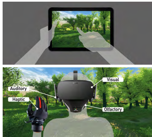
Figure 6. (top) The user interacts with the VR scene through a tablet; and (bottom) the user is immersed in the scene and provided with visual, auditory, haptic, and olfactory devices. The virtual scenes were created by the authors.
