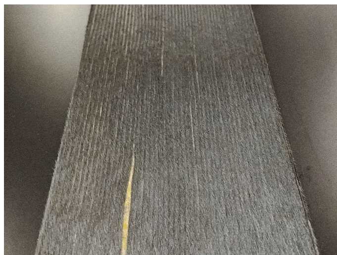
Figure 1. AFFT™ prepreg tape made with highly oriented reclaimed carbon fibers.
