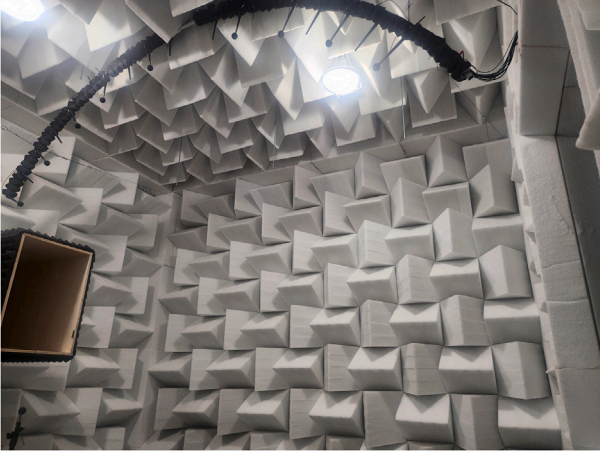
Fig. 5. Internal view of the anechoic test chamber of the POLIMI-DAER anechoic wind tunnel.
