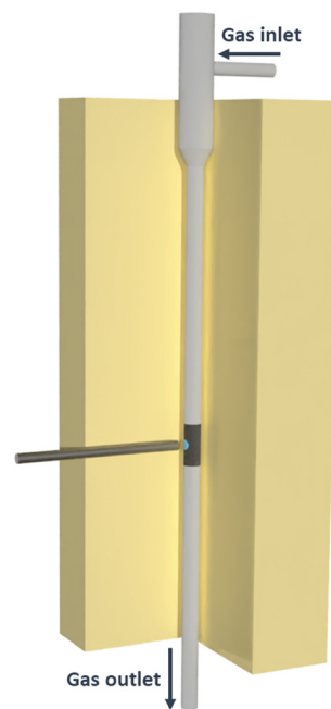
Fig. 1 Pictorial representation of the developed operando UV-vis setup combining the packed-bed reactor and the UV-vis probe.
