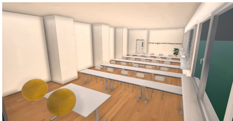
Fig. 7 View of the simulated room according to [91]. Users can select each chair in the room, the sources are depicted as two yellow spheres
