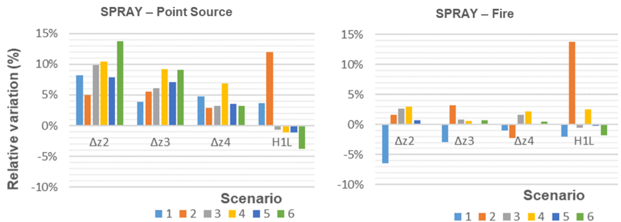
Figure 17. % variation of the maximum PM concentration values at the selected receptors resulting from the simulations of the alternative cases for model specific parameters of SPRAY – point source (left) and SPRAY – fire (right) compared to the reference base-case
