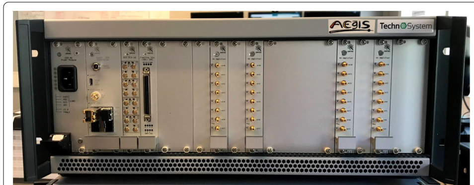
Figure 1 Photograph of one of three fully equipped Sinara electronics crates of the AEgIS trap control system, including (from left to right) power module, Kasli carrier, digital I/O units, Fastino DAC, and four high-voltage amplifier boards
