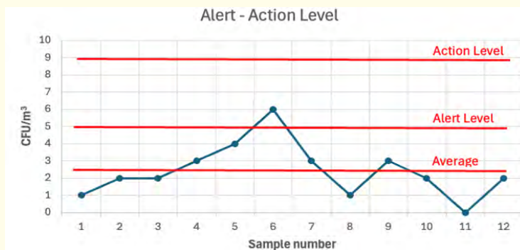
Figure 2: Example of alert and action levels. Limits should be set for each sample site and individual sample result should be evaluated against the action and alert levels.
