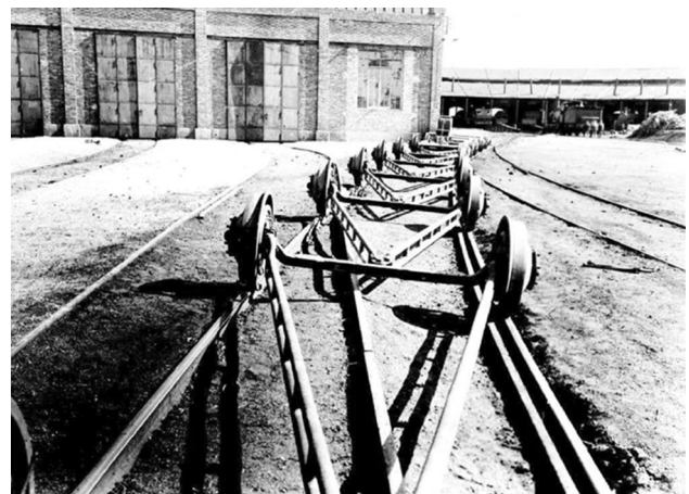
Fig. 28 Talgo solution of 1941 [106]
