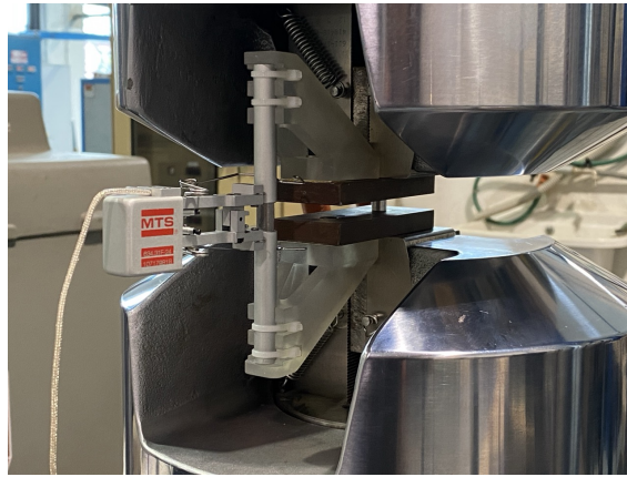
Figure 2: Compression test jig in use.
